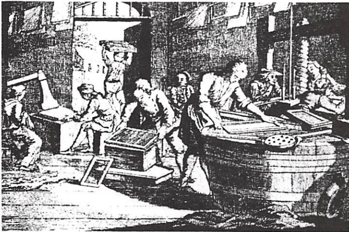
French paper mill showing the large wooden screw press for squeezing the water out of the newly made sheets, the “spurs” of paper being hung to dry and the large stone hammers (left) to polish each sheet.
