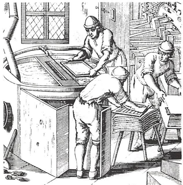
European Papermaking Showing the Vatman, Coucher and Layman at work
